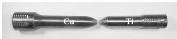
Figure 11 Base metal fracture after tensile test. (Upset time ( t_2 ) = 6 sec, Friction pressure ( P_1 ) = 100 MPa, Friction time ( t_1 ) = 0.7 sec and Upset pressure ( P_2 ) = 325 MPa.)
