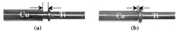
Figure 3 Appearance of copper-titanium joint. (a) Friction time ( t_1 ) = 0.1 sec, Upset pressure ( P_2 ) = 100 MPa and (b) Friction time ( t_1 ) = 0.1 sec, Upset pressure ( P_2 ) = 325 MPa.
